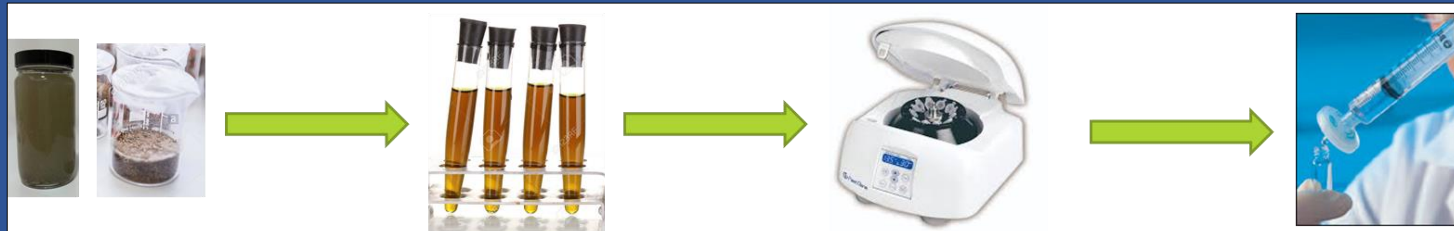
Figure 1: Phage extraction from environmental samples. Sample collection, incubation in broth, centrifugation and filtration.
